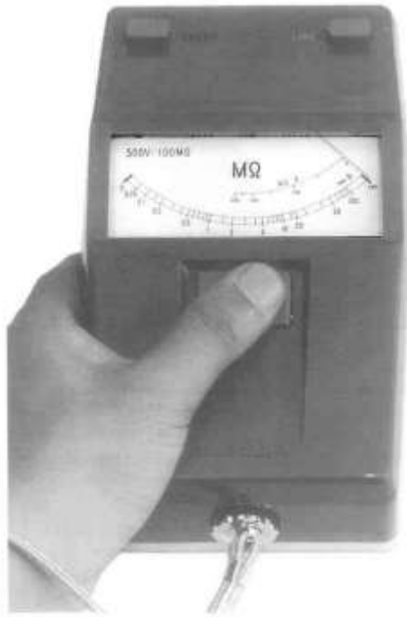
Fig. 11.15 This battery-operated insulation-resistance tester is light and compact
