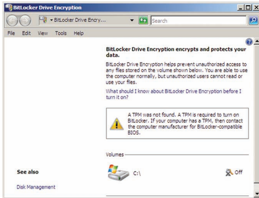
Figure 10-14 Warning for missing TPM chip
