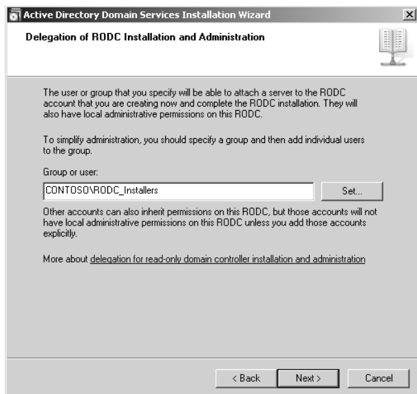
Figure 3-3 Delegating installation and administration of an RODC
