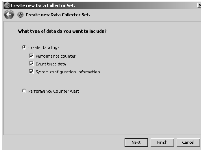
Figure 7-17 Creating a new Data Collector Set manually
