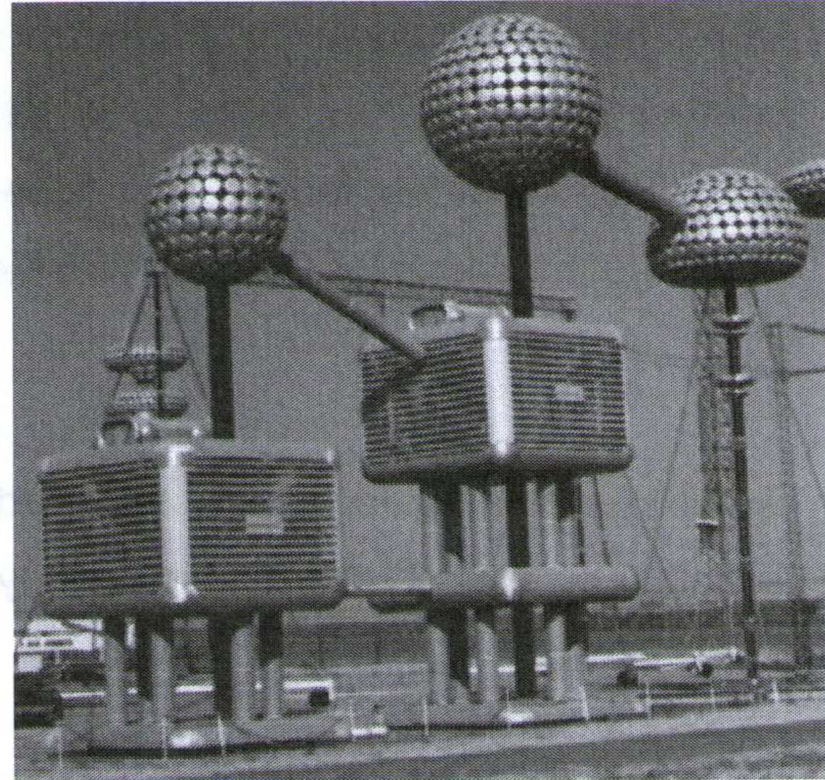
Fig. 4.3: Cascade connected test transformers
