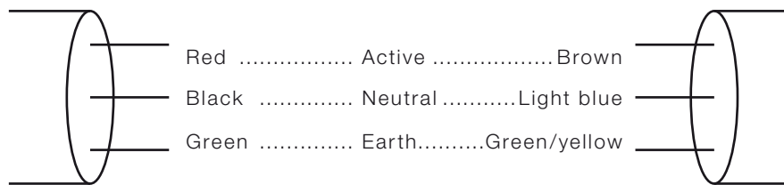
FIGURE 3.1 SINGLE-PHASE CABLES
