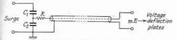
FIG. 268. POTENTIAL DIVIDER AND DELAY CABLE
