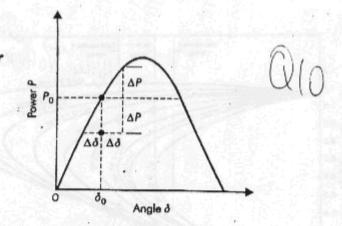
Figure : 2 Small disturbance—initial operation on power-angle curve at  $P_0, \delta_0$ . Linear movement assumed about  $P_0, \delta_0$
