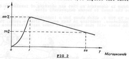
The wave specification of 1/50 indicates that the test voltage rises to the peak value in lusec and then drops to 50% of the peak value by  $50\mu sec$ .
