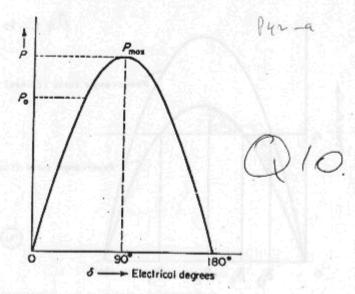
Figure 1 Power-angle curve of a synchronous machine. Resistance and saliency are neglected
