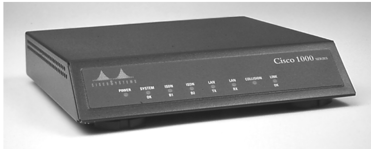
Figure 2-4 Cisco 1000 Series Router
