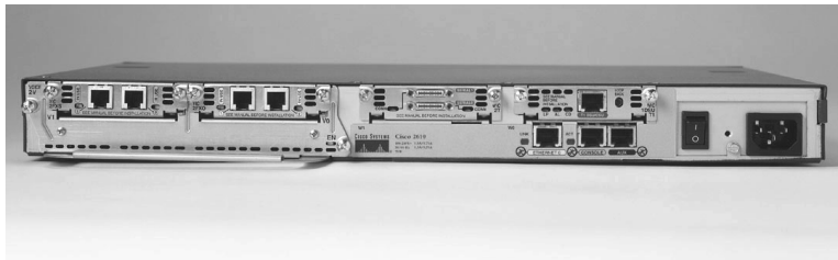
Figure 2-7 Cisco 2600 Series Router
