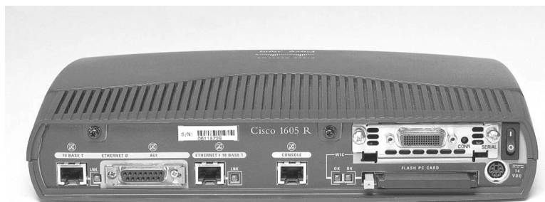
Figure 2-5 Cisco 1600 Series Router
