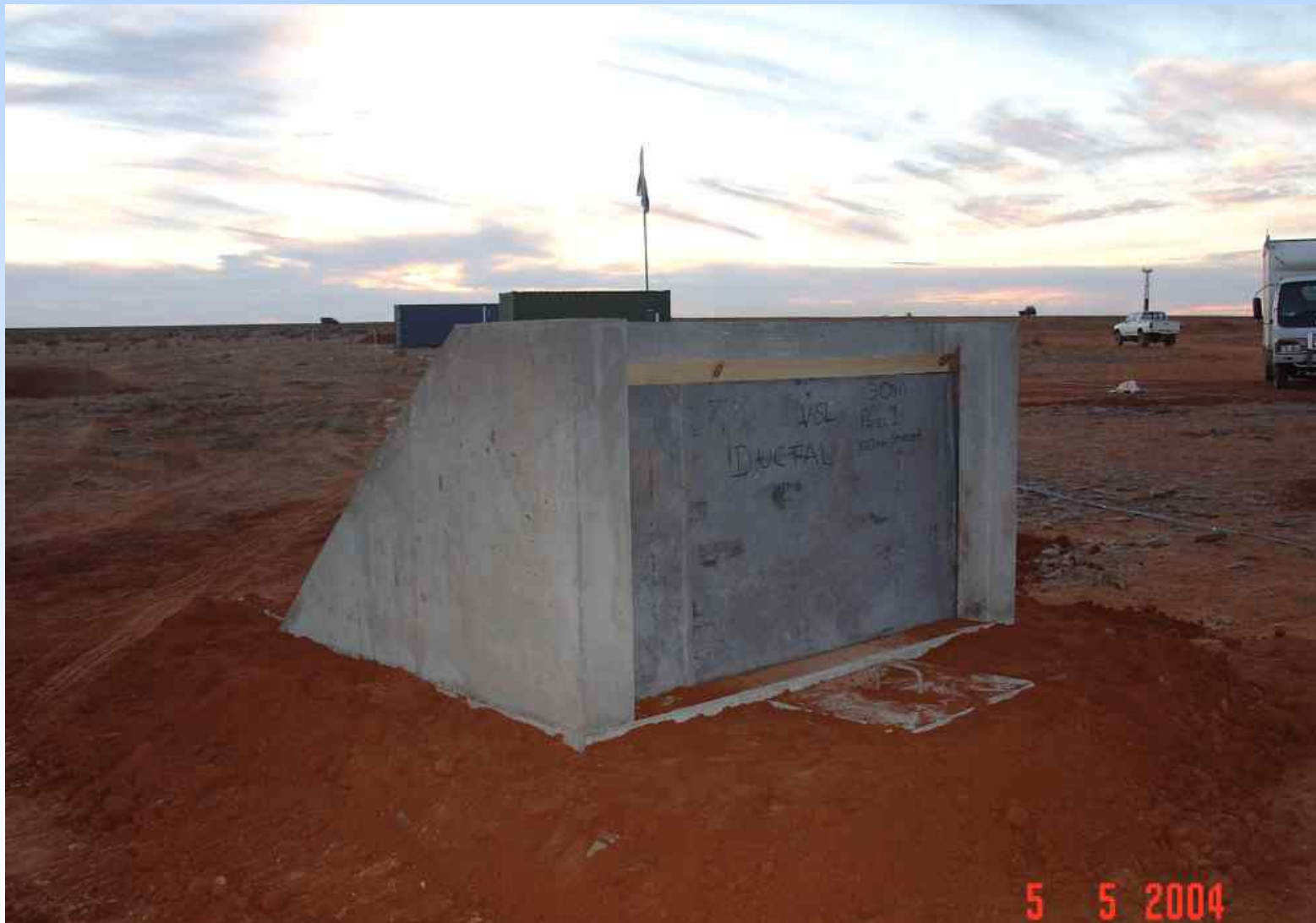
BLAST 1 - 100mm stressed at 30m; ready for blast test
